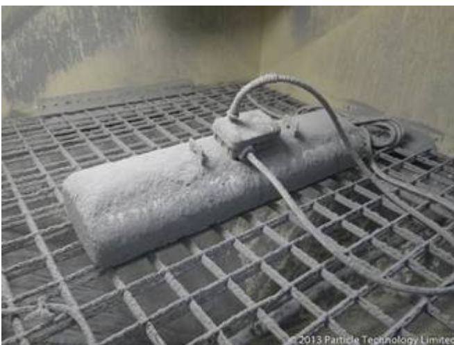
Figure 1 – HLW 15 after IP6X dust test
